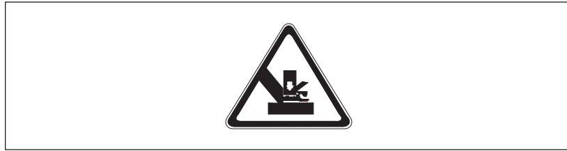
Figure 2-5. The pinching hazard label.
